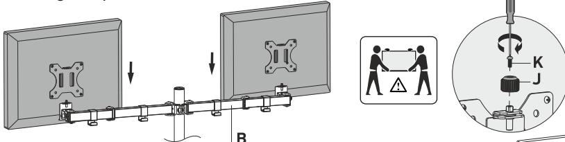
**4b.** Install your screens at a desired angle and turn the key (N) clockwise to tighten the screw. In order to set another angle just loosen the screw a bit.
