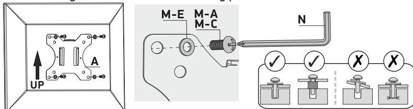
Other screws (M-B), (M-D), washers (M-E) and spacers (M-F) can be used as required. You may use the key (N). Make sure VESA panels are securely fixed. Take a good look at the following picture:
