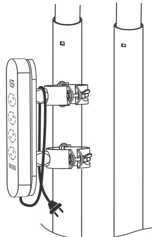
Wind the wires on the legs of the holder in case of transportation. There is no need to take it off the stand.
