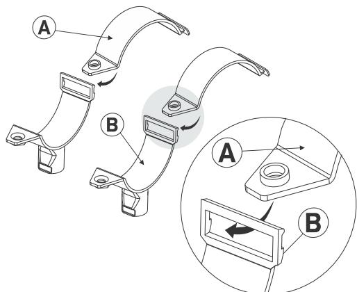
**2** Grab the tube with half-rings and connect them together with screw and nut. Make sure that half-rings are not completely tightened.
