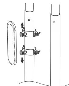
**5** Peel off the top layer of the adhesive tape.
