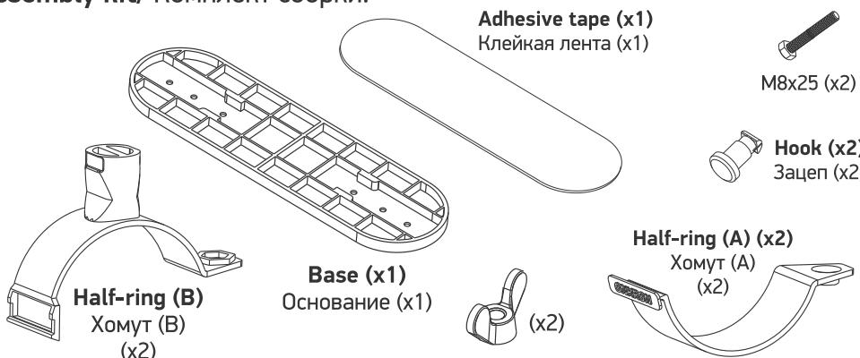
**1** Put half-ring (A) through the hole in half-ring (B). Repeat for half-ring (A).
