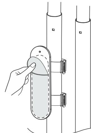
**6** Press firmly power strip to the base of the holder. Now power strip is securely fixed.
