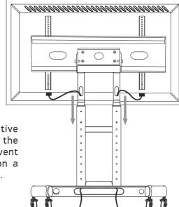
Put cables through protective rings before connecting the touch panel / TV. They prevent cables from scratching on a sharp edge of the columns.
