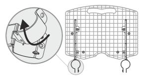
• Tighten bolts (1) and (3) using a screwdriver.
