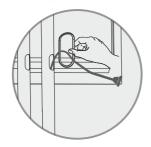
Put protective rings into cable management holes in the columns.
