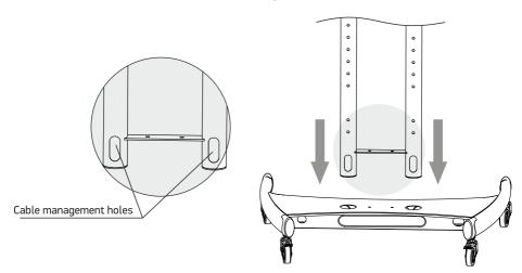
• Use key (I) to attach the columns to the base with bolts and washers (F) from above.
